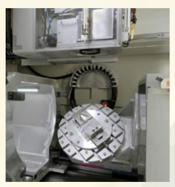
圖2:激光抛光設備工作平台(德國Fraunhofer ILT 提供) Fig.2: Platform of laser polishing machinery (courtesy of Fraunhofer ILT, Germany).
