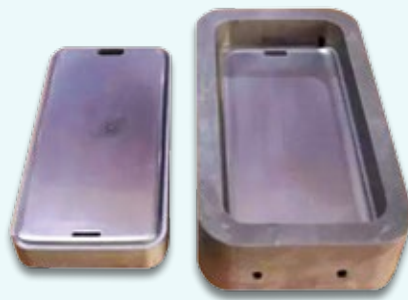
圖一 3D玻璃用石墨模具 (kknews) Figure 1 Graphite Mold for 3D glass (kknews)
