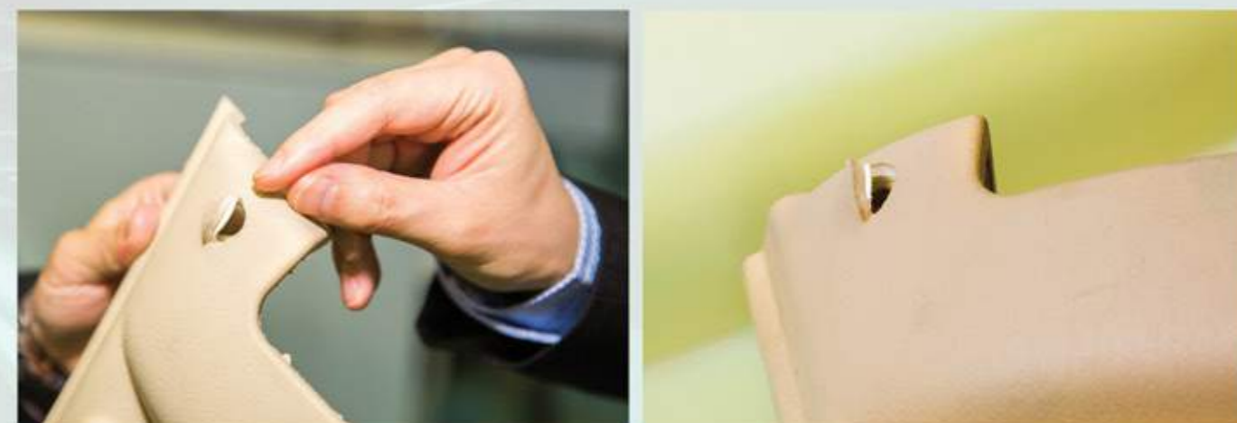
研發團隊經過反覆的測試，確保PU橡膠與汽車內側門板的ABS塑料底材，兩者牢固地黏合。 Repeated tests on the door trim to ensure PU has good adhesiveness with ABS substrate.
